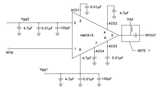
NOTE 1: Drain Bias (Vdd) must be applied through a broadband bias tee with low series resistance and capable of providing 500mA
